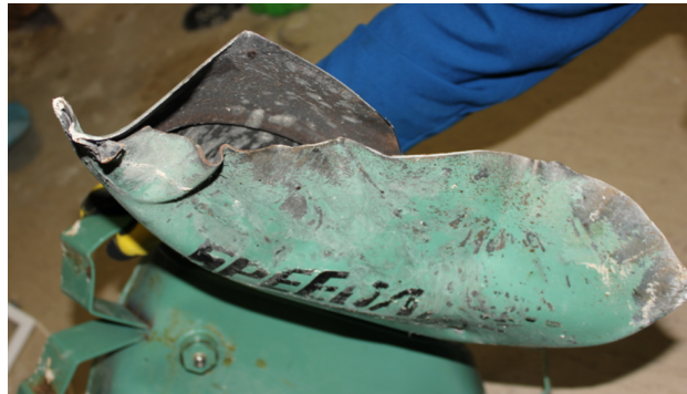
Figure 10: Damage to a -20°C refrigerator and freezer doors in the POST 30 laboratory. The doors show severe impact damage by the gas storage tank piece shown below. The paint residue on the doors match the tank's paint.
