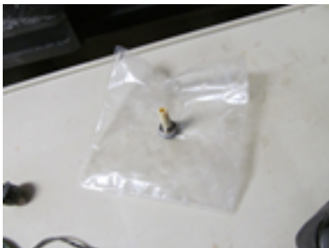
Figure 6: Gas sampling bag found in the UH laboratory with polyethylene tubing attached.
