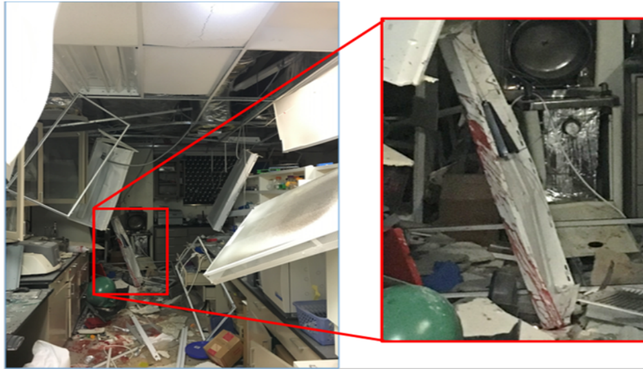
Figures 18 and 19: Photographs taken during HFD 48 response of the explosion scene with torn down ceiling plates and light fixtures. Both pieces of the tank landed to the left of the Biosafety Cabinet. The autoclave with its lid open is visible in the background. Blood from the injured postdoctoral researcher is visible in various places. The inset shows a ceiling light panel from in front of the biosafety cabinet that was impacted by the ball valve assembly and a remnant of the gas storage tank (green) can be seen in the lower left corner.
