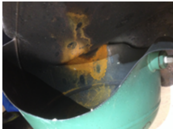
Figure 5: Rust inside the damaged gas storage tank as observed by the Investigative Team.
