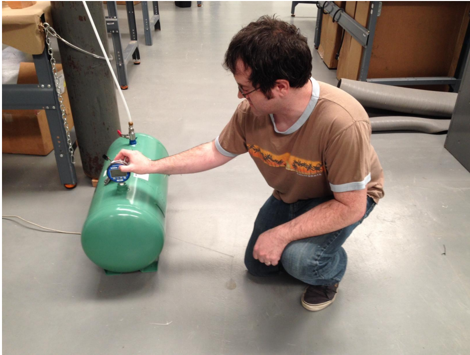
Figure 31: WHA engineer testing static electricity discharge by simultaneously touching the pressure gauge housing and pressing the gauge's On/Off switch
