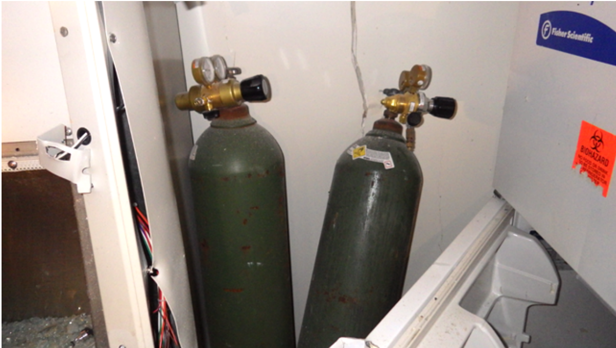
Figure 21: Oxygen cylinders used to fill the gas storage tank (standing upright) and used for the second postdoctoral researcher's ongoing experiment (tilted). The latter oxygen cylinder was open at the time of the explosion.
