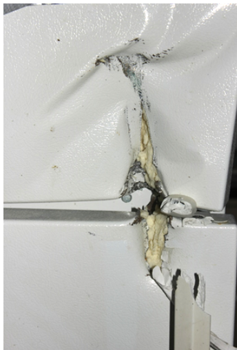
Figure 10: Damage to a -20°C refrigerator and freezer doors in the POST 30 laboratory. The doors show severe impact damage by the gas storage tank piece shown below. The paint residue on the doors match the tank's paint.
